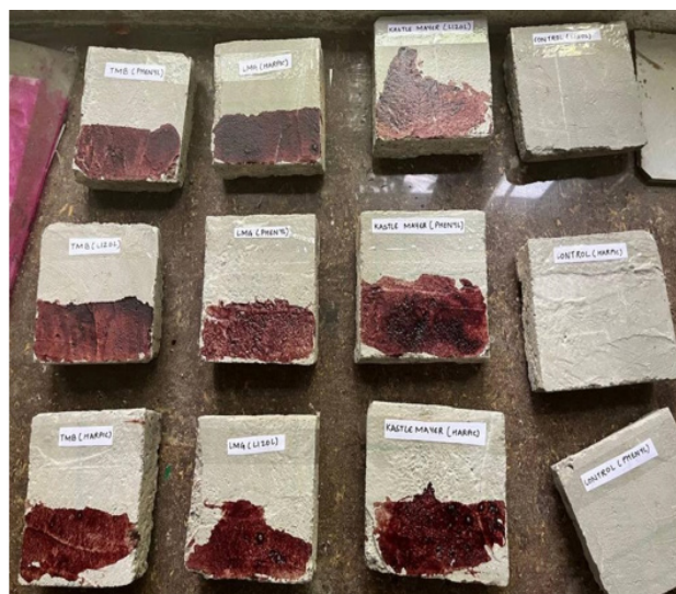
Fig. 3 Concrete surfaces labelled and stained with blood along with control samples.
